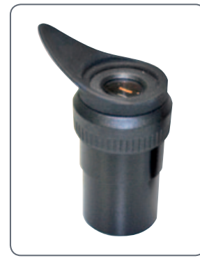
Fixed eyepiece with inclined eyecup.
